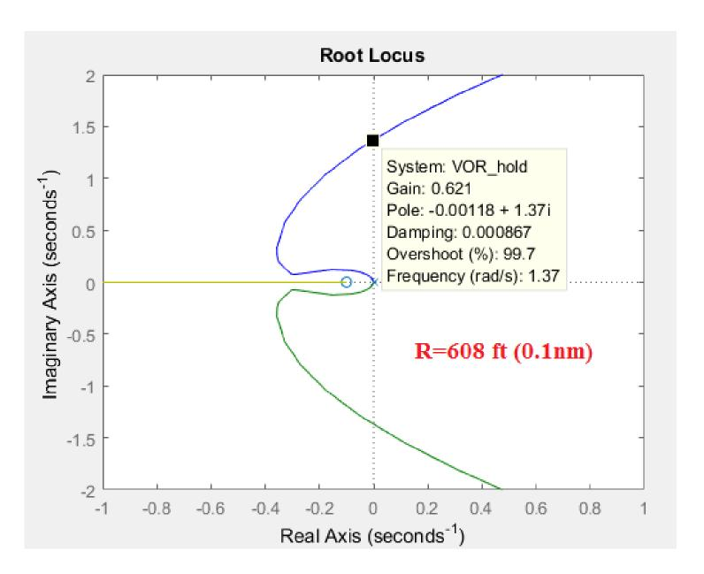
• The VOR hold loop root locus diagram for this case in shown in figure . Operating points are shown for R=50nm, R=5nm and R=1nm.. This system works well for this airplane even without adjustment to the coupler gain as a function of slant range. Note however, that the constant coupler gain the closed loop damping ratio greatly diminishes as the airplane approaches the VOR transmitted. The behavior is typical of constant gain loops.
