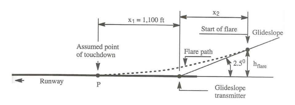
Assume that the flare path can be approximated by a relation which makes it tangential to a point P
