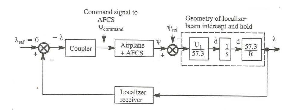
Figure .2 shows a block diagram corresponding to the localizer hold system
